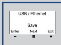
3. Note: once the Ethernet port is enabled, the USB port will be disabled.
