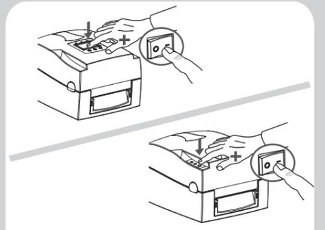
Press and hold the FEED button then power on the printer. After the printer beeps 3 times, release the FEED button and a Self-test label will print.
